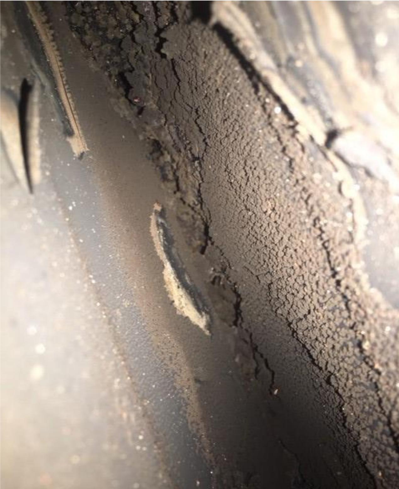
Picture above: This is a close up of the left most flue gas passage way. This is caked on soot that accumulated on the walls of the heat exchanger and completely plugged this passage. For normal operation this needs to be totally unrestricted.
